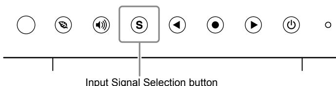
Switch the input signal with **(S)**. Input signal switches each time **(S)** is pressed. When the signal is switched, the active signal type (Analog or Digital) appears at the top right corner of the screen for three seconds.
